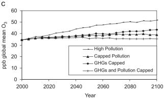
Fig. 1. Global changes in temperature, CO<sub>2</sub> concentrations and ozone levels: (a) temperature change; (b) CO<sub>2</sub> concentration; and (c) ozone level.
